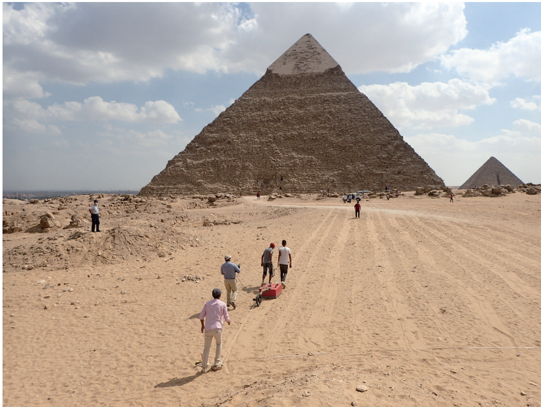
Fig.3 The GPR Survey at the Western Cemetery
